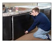
Unscrew and remove the front cabinet panel.
